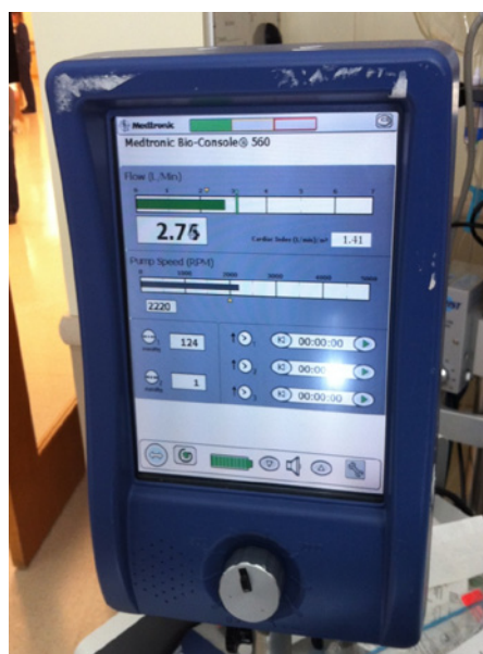
Figure 4: Control monitor to adjust flows and to monitor cannula inflow/outflow pressures.
