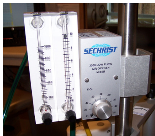
Figure 5: Gas blender (left) to control "sweep" to eliminate carbon dioxide (CO 2 ) and to adjust oxygen support (right).
