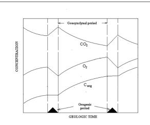
**Figure 2:** Natural redox carbon cycle model. The scheme of the putative variations of  $CO_2$  and  $O_2$  in the "atmosphere – hydrosphere" system and of organic carbon accumulation in sedimentary rocks in the course of orogenic cycles. Note that according to photosynthesis reaction, the variations of  $CO_2$  and  $O_2$  are anti-phase, while the variations of  $O_2$  and organic carbon Corg are in phase.
