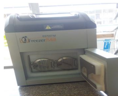
Figure 3: Model of liquid nitrogen DNA bone grinding machine.
