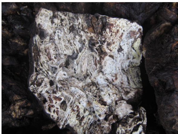
Figure 2: A cut portion of rubber lump to checkmate adulteration
