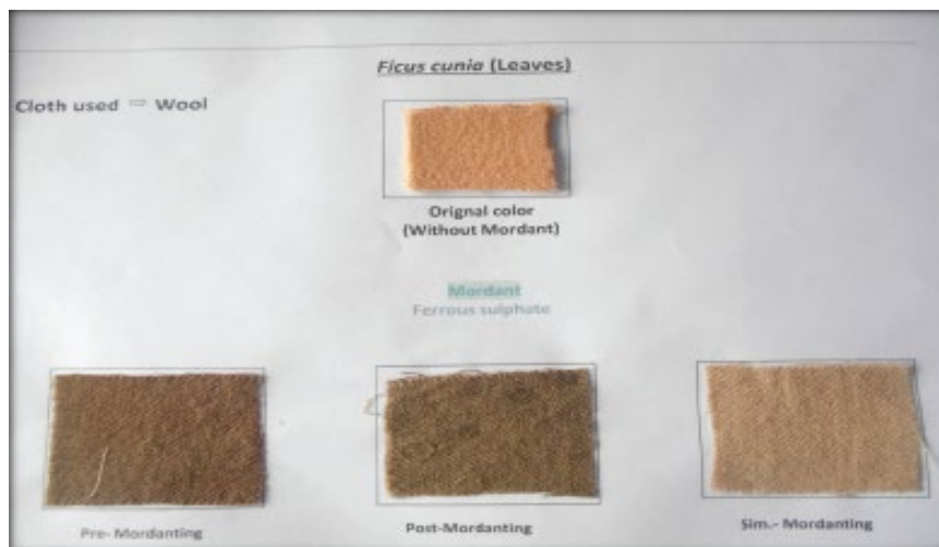
Photograph 7: Shows effects of various shades obtained from different mordants and mordanting methods.
