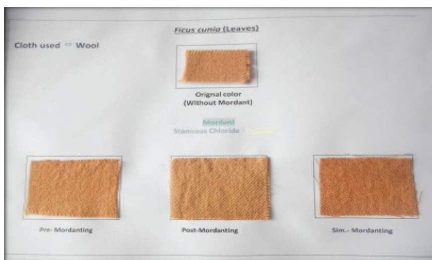
Photograph 8: Shows effects of various shades obtained from different mordants and mordanting methods.
