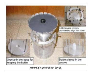
cone can fall straight into the bottle and the falling droplets can be seen. Depending on prevalent relative humidity, it takes 30 minutes to 60 minutes for collecting 5 to 10 ml of liquid condensate. However, during the rainy season when relative humidity is very high, the sampling bottle is filled even within 30 minutes. After setting up the conical condensation device the date, time, temperature and relative humidity are recorded using thermo-hygrometer [29].
