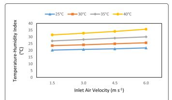
**Figure 15:** The temperature-humidity index effectiveness at different ambient temperatures and inlet air velocities.
