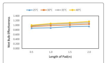
**Figure 8:** The wet bulb effectiveness at different ambient temperatures and lengths of pad.
