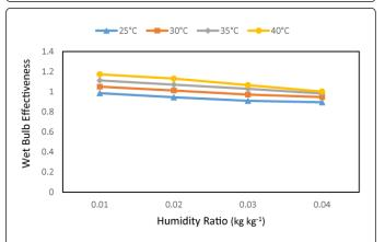
**Figure 7:** The wet bulb effectiveness at different ambient temperatures and humidity ratios.
