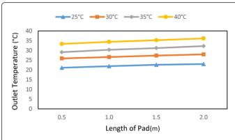
**Figure 5:** The outlet temperature at different ambient temperatures and lengths of pad.
