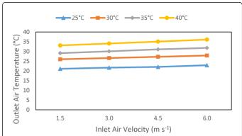
**Figure 3:** The outlet temperature at different ambient temperatures and inlet air velocities for the direct evaporative cooling system.
