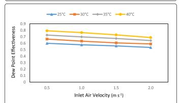
**Figure 9:** The dew point effectiveness at different ambient temperatures and inlet air velocities.
