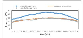
**Figure 18:** The predicted and the measured outlet temperatures of evaporative cooling system.
