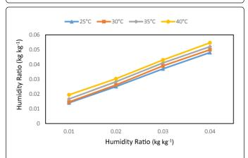
**Figure 13:** The humidity ratio effectiveness at different ambient temperatures and humidity ratios.
