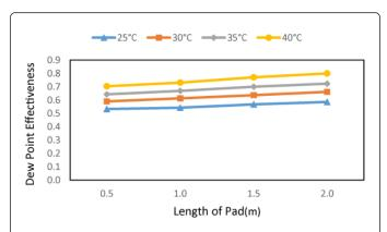
**Figure 11:** The dew point effectiveness at different ambient temperatures and lengths of pad.
