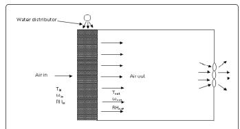
**Figure 1:** The input and outputs of the heat and mass balance of evaporative cooling system.
