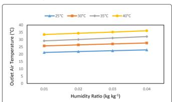
**Figure 4:** The outlet temperature at different ambient temperatures and humidity ratios.
