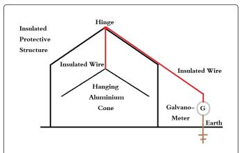
Figure 3: Cross-section of a suggested circular apparatus to detect charged vapor up-flux coming off desert-sand.
